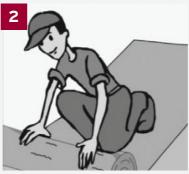
Lay the Floover film on the ground and seal with a masking tape to ensure the vapou barrier.
