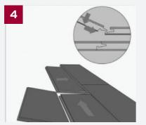
Install the following rows introducing the short side with 45° and laying on the floor with low pressure.
