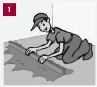
The floor must be levelled not over 2 mm
