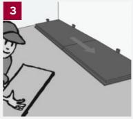
Install the first row following the direction of the sun Light, respecting the 12mm gap with all the walls and elements. Join the plank with Unilin clic system.
