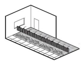
1. Moisten well the surface to be covered .Loose lay the tiles, making sure joints and studs are correctly aligned; check the uniformity of the colour and the absence of defects.
