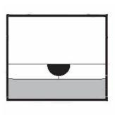
**4.** When the rod has cooled to roomtemperature the remaining excess shouldbe trimmed using the spatula knife withoutthe guide keeping a shallow angle betweenblade and floor to avoid "digging in". Attention: the colour of the rod cannot be exactly the same of the floor.
