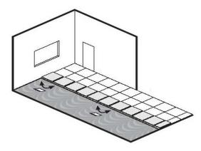
**4.** Tip over a row of tiles at a time. Spreadthe adhesive with the proper notchedtrowel as advised by the manufacturer..
