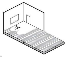
Apply the permanent tackifier with a notched trowel in accordance with the instruction of the manufacturer. Allow theadhesive to dry sufficiently.
