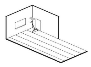
**3.** After the laying, the use of a floor roller is recommended to ensure a perfect contact with the substrate.
