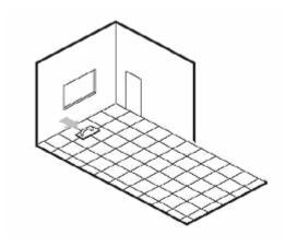
**3.** Prepare a liquid mortar of cement 325 and water and spread iton the screed. Lay the tiles back in the starting position and fit them with a trowel. Press/massage the tiles to make sure thaall air is expelled and the tile is in full contact with the substrate; let the exceeding mortar come out from joints.
