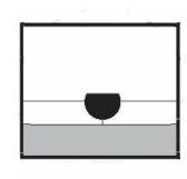
Using a sharp spatula knife placed on atrimming guide and trim off the first partof excess sealing rod. Heating the knifewith the sealing gun may help thetrimming.
