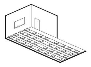
**4.** In case adhesive with long tackifying time are used, apply weights along the joints (bricks, sand bags, etc.).
