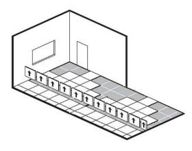
**2.** Loose lay the tiles (without adhesive)starting along the centrelines and following the arrows printed on the back of the tile staking special care to the alignment of joints and/or pattern.
