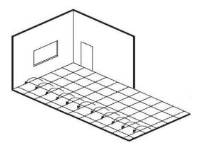
**5.** Once the adhesive is ready to accept the tiles, put the tiles back in the starting position. Press/massage the flooring to make sure that all air is expelled and the tile is in full contact with the substrate.
