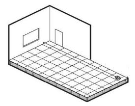
1. Measure the room and mark the centrelines planning the laying in a way to reduce cuts and scraps.
