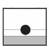
2. Place the sealing rod into the speedweldaperture, press the rod down into the groove and proceed at the right speedkeeping the speedweld toe parallel to therubber surface.
