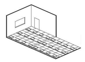
**6.**Special care has to be taken with regards to the positioning of the tiles to make sure the alignment of joints and studs is accurate. In case adhesive with long tackifying time are used, apply weights along the joints (bricks, sand bags,etc.).
